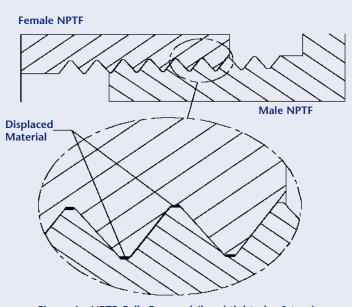
Figure 4 – NPTF, Fully Engaged (hand tight plus 1 turn)
