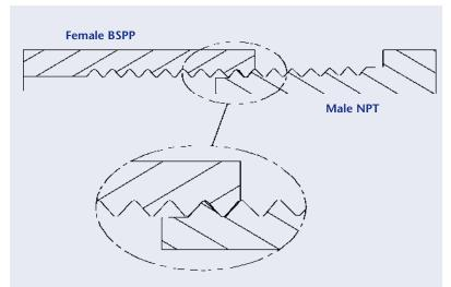
Figure 5 – Male NPT in a Female BSPP with Different Pitch
